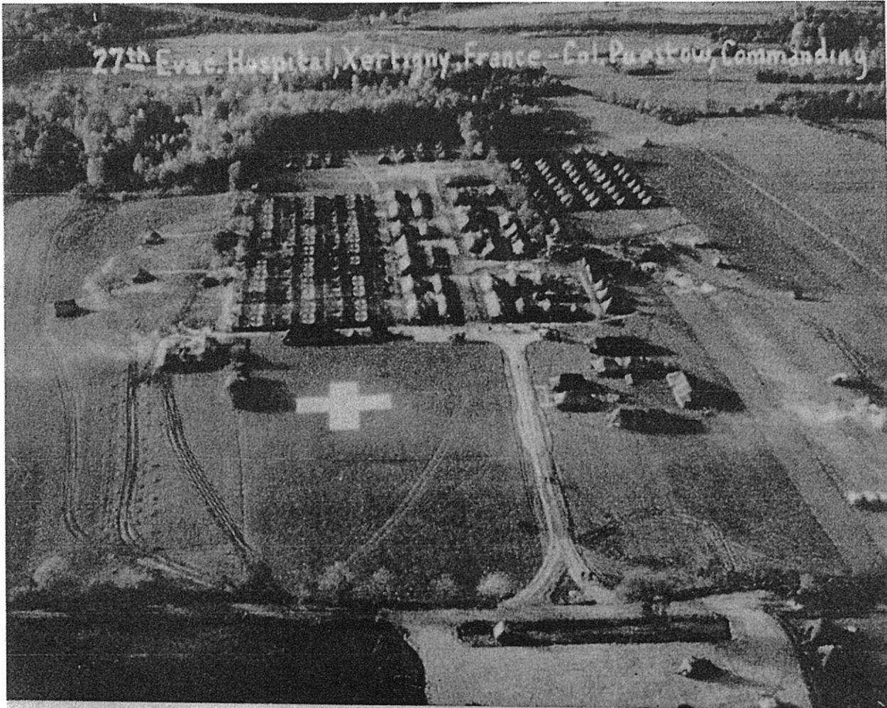
This was a most satisfactory arrangement of tents. Three ward tents end-to-end formed a ward accomodating up to 75 patients
